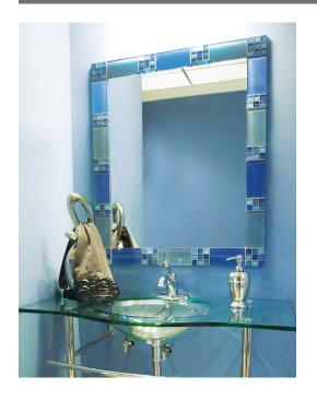
Glass tile will adhere to mirror / glass and mirror will adhere to wall with Spray-Lock® Wall Tile Adhesive! (As shown in photo)
